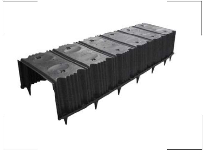
U-Bahn<sup>®</sup> Beton is a modular framework in recycled polypropylene that was specifically designed to create one way slabs that are cast on site or semi-prefabricated. The various elements, overlapping in their terminal sections, allow the creation of ribs of any length.
