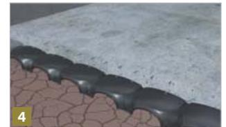
4 Casting of the reinforced concrete to form a load-bearing slab that is reinforced and supported with a cavity along the edges to accommodate the movements of the ground.
