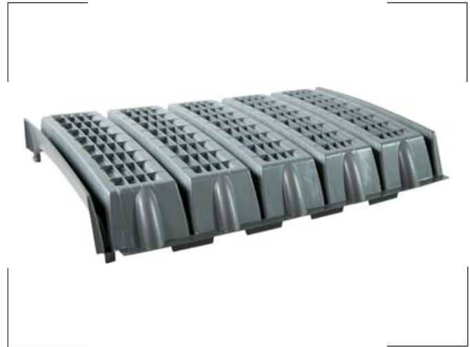
**Fit Slab** is a formwork made of polypropylene; its principal function is lightening and, when used in conjunction with prefabricated beams made of pre-stressed reinforced concrete, or lattices or directly on prefabricated lattice slabs, it enables the construction of various types of voided slabs made of reinforced concrete, with extremely quick installation in both reconstructions and new buildings.
