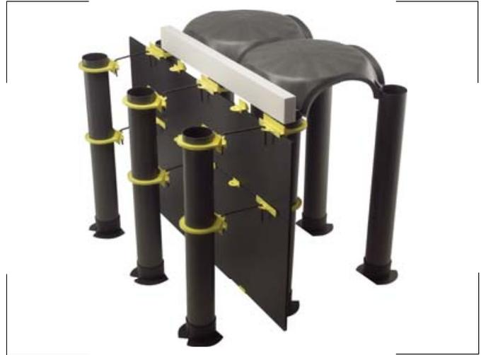
Cassaforma Muro (*Wall Formwork*) was designed as an alternative to traditional wood shuttering, which permits casting walls at a height, reversed beams and foundation bases, drastically reducing the time for creating the foundation. This disposable formwork consists of a combination of pipes, panels, collars and stirrups all made of polypropylene.
